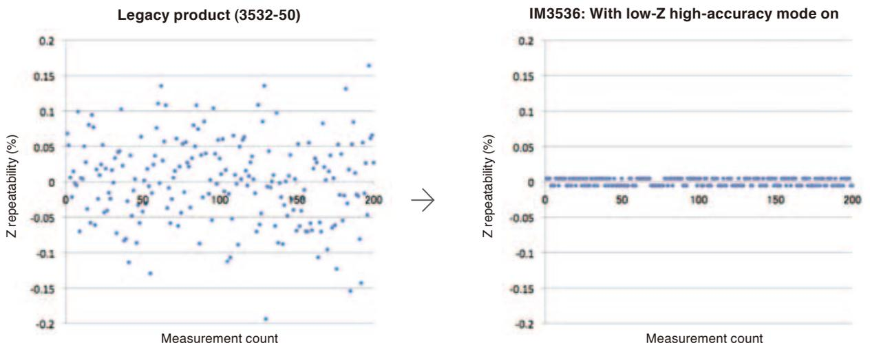
Graphs illustrate the results of measuring a resistance of 1 mΩ 200 times under the following conditions:
