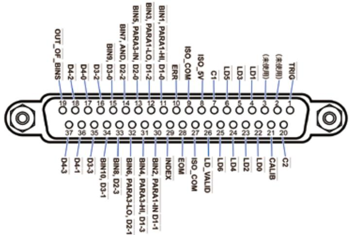
Signal assignment is different during continuous measurement mode. Signal logic is 0 V to 0.9 V for LO level and 5 V to 24 V for HI level.
