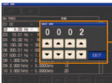
Number of waveforms → Many (increased measurement precision)
