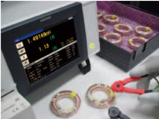
Save 32000 measurement results, copy them to a USB flash drive, and load them onto a computer. You can then open the measurement data using a spreadsheet to analyze variations and manage test data.
