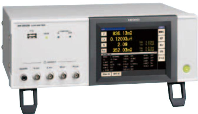
*This product is not supplied with measurement probes or test fixtures. Please select and purchase the measurement probe or test fixture options appropriate for your application separately. All probes are constructed with a 1.5D-2V coaxial cable. For an RS-232C connection: A crossover cable for interconnection can be used. You can use the RS-232C CABLE 9637 without hardware flow control.*
