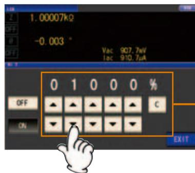
The judgment standard is calculated based on the measurement range and judgment reference value (valid setting range: 0% to 30,000%).
